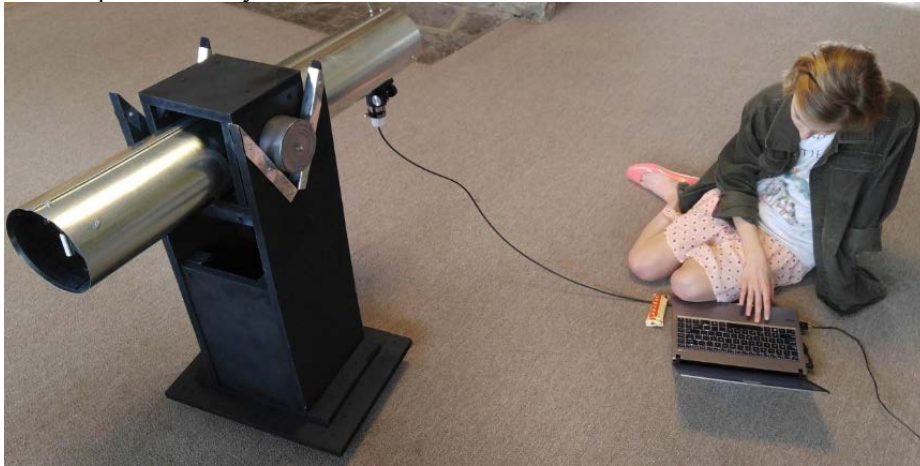
Fig. 2. This near-infrared telescope for SETI uses all gold first surface optics and a high speed InGaAs detector. An SDR connects the detector to the computer for data monitoring and collection.
