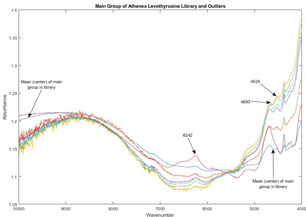
**Figure 11.** The mean spectrum of the main group in the library (i.e., center) is shown as a blue spectrum and marked at each end. In the main group of spectra, the peak at  $4693\text{ cm}^{-1}$  is bigger than the peak at
