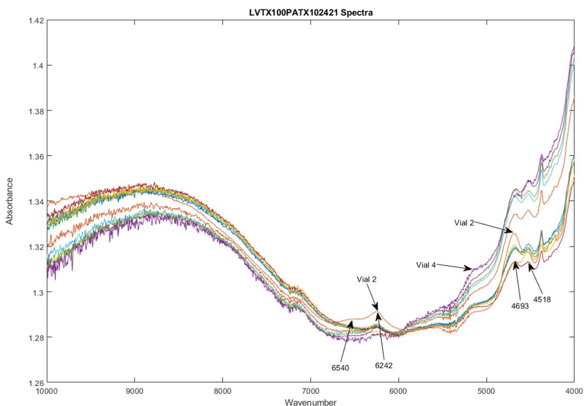
**Figure 1.** Spectra of 12 vials of levothyroxine from Lot AFN102. Two vials (numbers 2 and 4) are flagged as unusual, due in part to the changes in relative intensity of the signals at 4518 and 4693  $\text{cm}^{-1}$ . A zoom-in on this region is provided in Figure 4. The appearance of more noise than usual in the spectra is due to the comparatively low amount of drug in the vials (100  $\mu\text{g}$ ).
