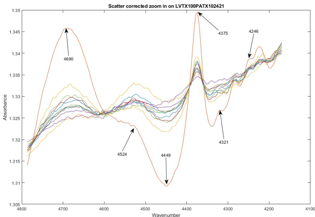
**Figure 4.** Zoom in on the spectra in Figure 1 in the region from 4100-4800  $\text{cm}^{-1}$ . The spectra were scatter-corrected across this region for the figure. The orange line that is labeled with wavenumbers is vial 2.
