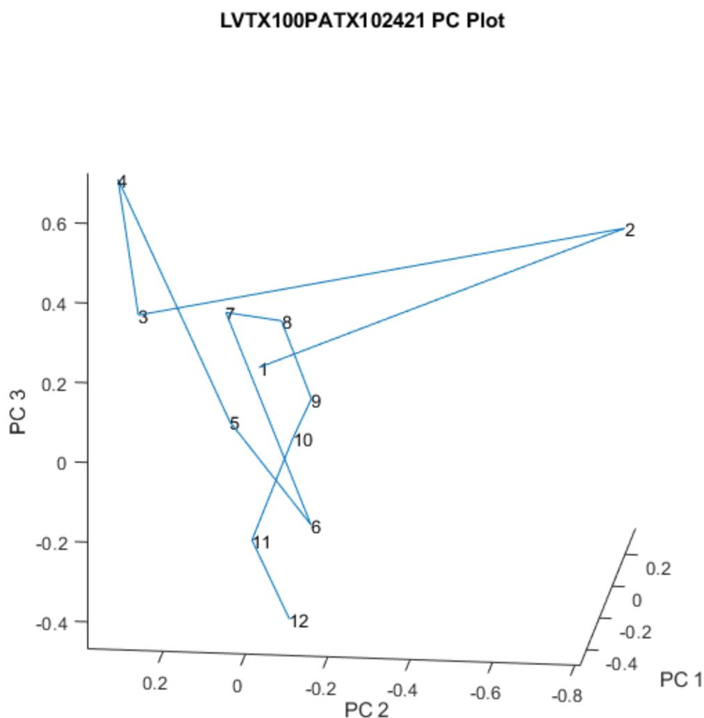
**Figure 2.** Principal components of spectra of 12 vials of levothyroxine from Lot AFN102. Two vials (numbers 2 and 4) are flagged as unusual, but vial 2 sticks out more than vial 4 in this view. Rotation of the axes produces Figure 3, in which both vials 2 and 4 appear as outliers (10.1 and 9.1 SDs from the center of the cluster, respectively).
