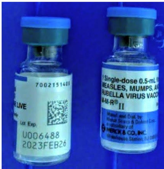
**Figure 14.** Photograph of MMR vials. Spectra were collected using diffuse reflectance from the lyophilized cake through the bottom of the vials.
