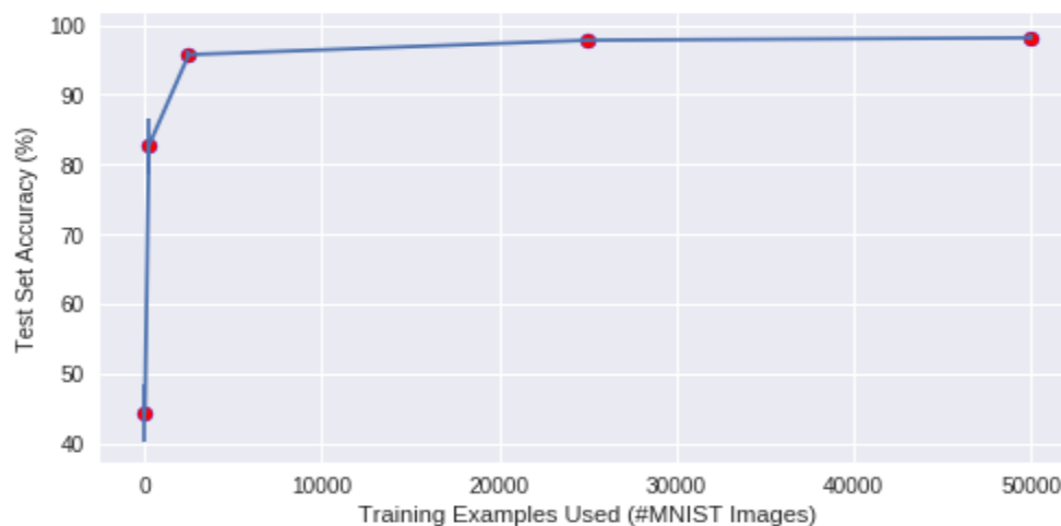
Figure 2. Effect of MNIST Training Set Size on MNIST TestSet Handwritten Digit Recognition of CNNs (n = 10 x CNNs per Group)
