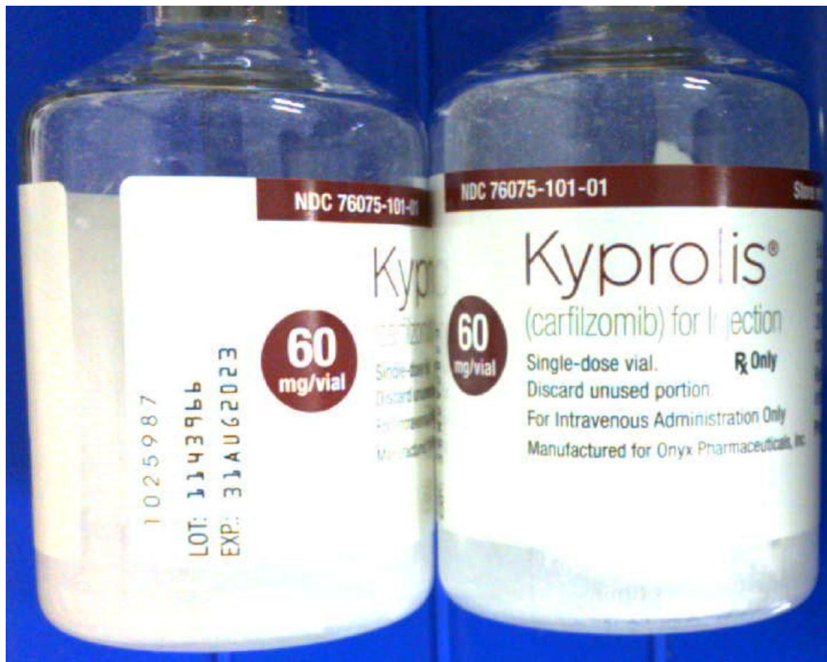
Figure 1. Vials of Kyprolis®(carfilzomib) for injection from lot 1143966. The drug appears as a white to off- white freeze-dried powder or cake. The vials were scanned nondestructively in the near-infrared spectral region through the bottom of the vials.
